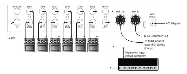
In this basic 6 pedal configuration, all you need to do is connect each loop send to a pedal input, and each loop return to the same pedal's output. Then, connect your guitar, amp and MIDI controller and you're ready to go!
